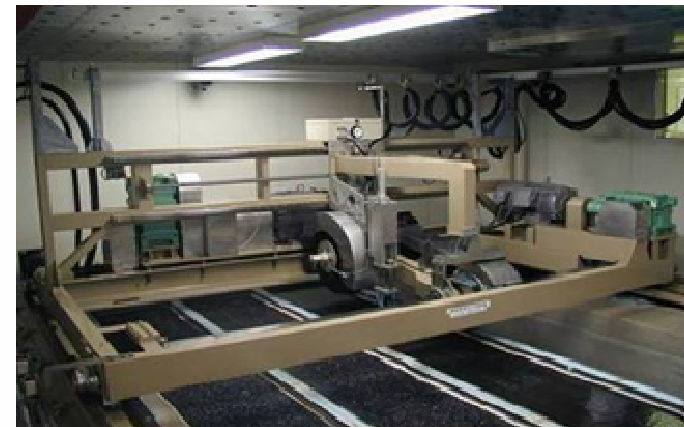
“Laboratory wheel-tracking test machine on ice”
