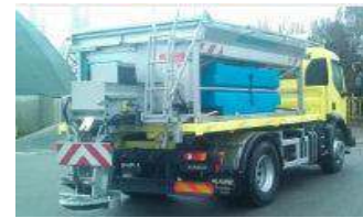
Lateral brine tank
