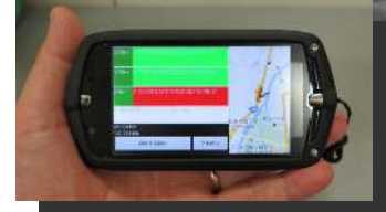
Friction data provided to operators on the spreader truck
