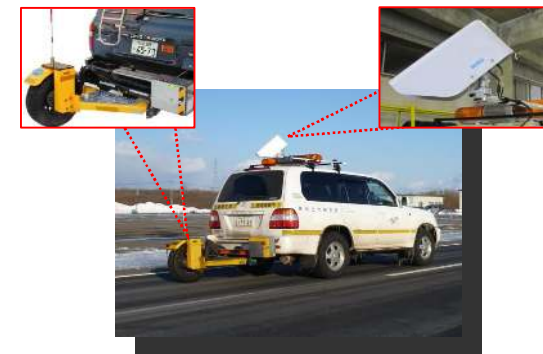
Vehicle Equipped with CFT and IR
