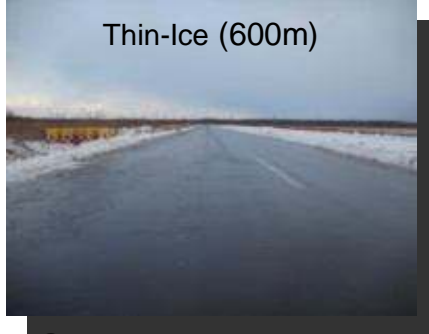
Road Surfaces Made on CERI's Test Track (Tomakomai City)
