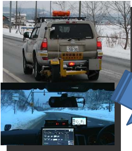
Real time friction values can be used to check road surface condition during patrol
