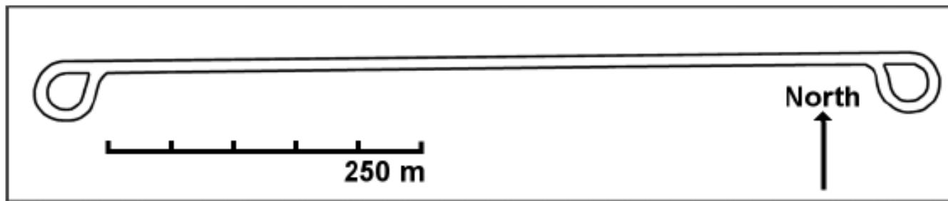
The field site consist of a ca 600 m long, 10 m wide test track with an RWIS-system (VAISALA Rosa) installed in the center position including four salt sensors (wheel tracks and in-between wheel tracks).
