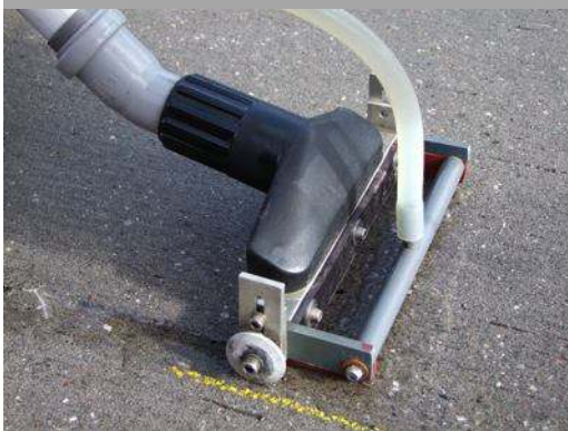
Suction port with pre-wetting nozzles
