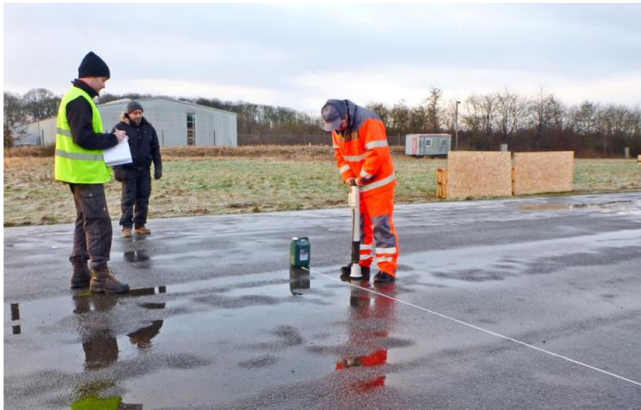
Figure 4 – Measuring residual salt with SOBO20 (old pavement).
