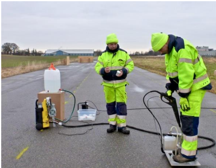
Figure 5 – Salt sampling with the Wet Dust Sampler (old pavement).
