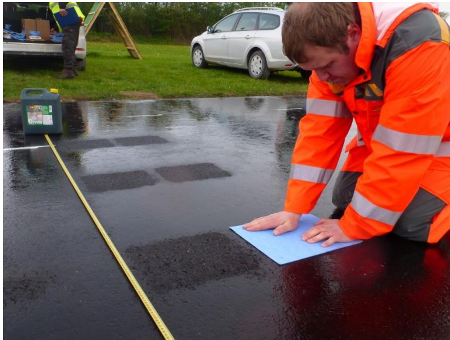
Figure 7 - Wetness as measured with the “Wettex”-method (new pavement).
