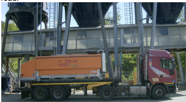
Figure 2 - Machine for the preparation and application of high-temperature pressurized solutions to the road.
