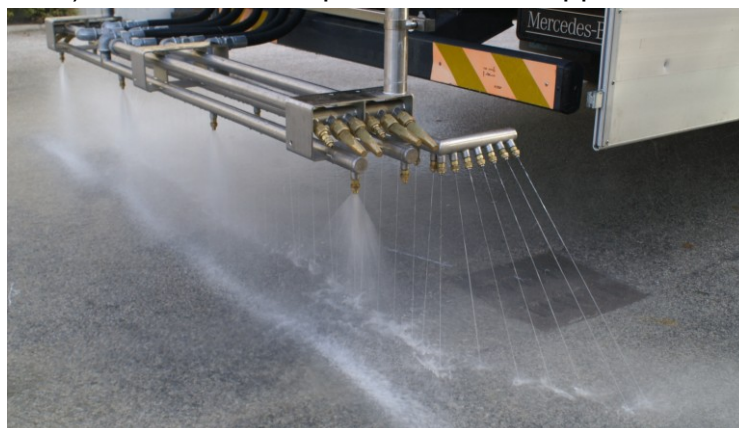
Figure 4 - Bar with rectilinear high-pressure jets
