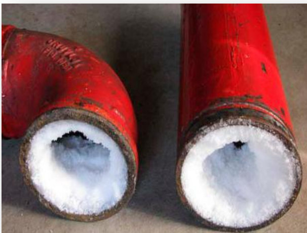
Figure 2 - Problem of ice plugs and corrosion in dry pipe system
