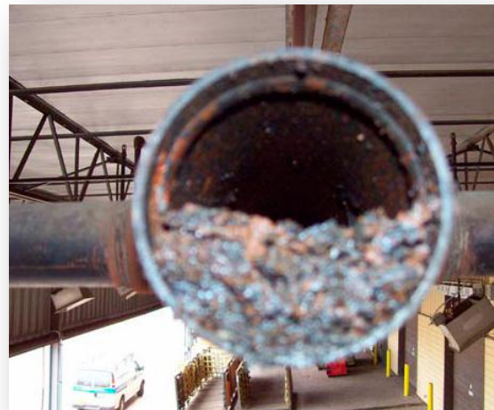
Figure 2 - Problem of ice plugs and corrosion in dry pipe system
