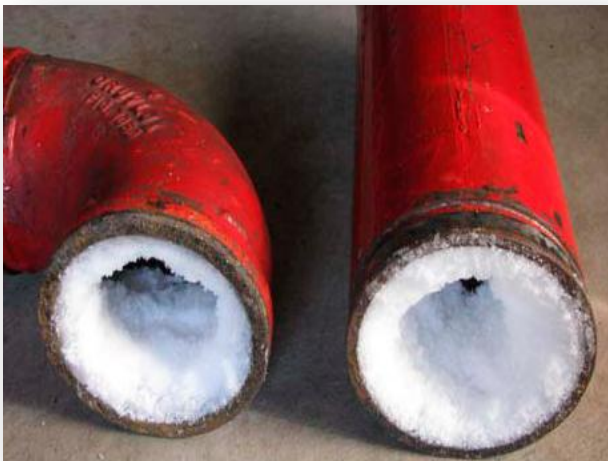
Figure 2 - Problem of ice plugs and corrosion in dry pipe system
