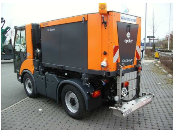
Picture 1 and 2: small and big liquid spreader for bicycle lanes and for motorways
