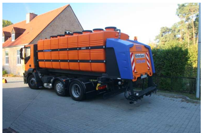
Picture 1 and 2: small and big liquid spreader for bicycle lanes and for motorways
