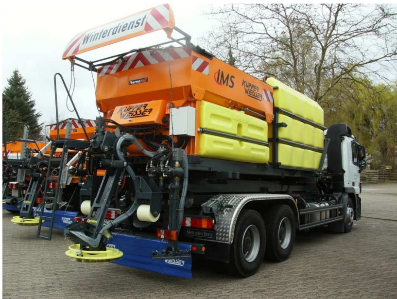
Picture 5: Big combined spreader for motorways with spreading disc and nozzles
