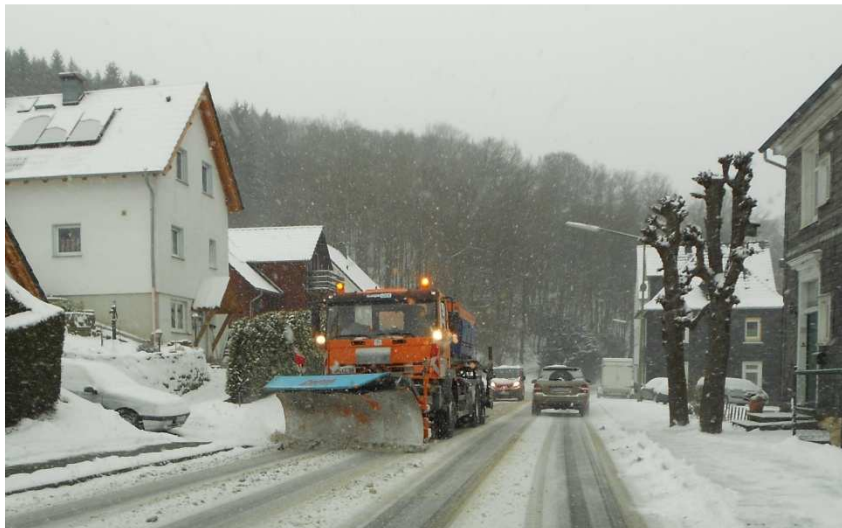
Picture 6: Spreading during snowfall
