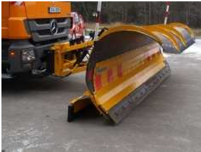
Picture 7: Example for aggressive plowing with double-blade snowplow
