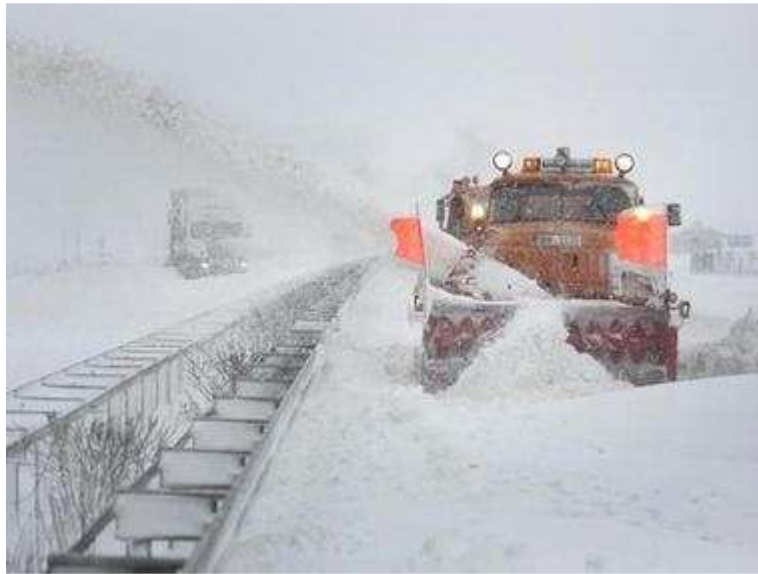
Picture 6: Snow removal machine with rotating tools on a German motorway
