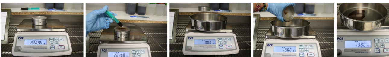
Figure 7: Process of testing liquid deicers in pictures with weighing, application of deicer using a syringe, exposure time, another weighing
