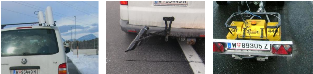
Fig. 15: Verification of film thickness and resulting skid resistance based on longitudinal measurements with (a) optical device #1 (Vaisala) (b) Optical device #2 (Teconer) (c) Skid resistance (Griptester MK II)
