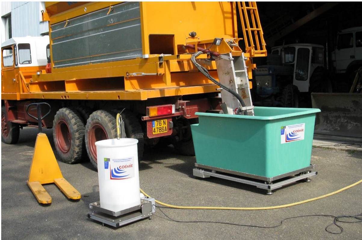
Photo 1 - Control of a spreader with the system
