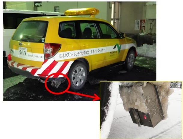
Figure 3 - Vehicle with the system and salinity sensor
