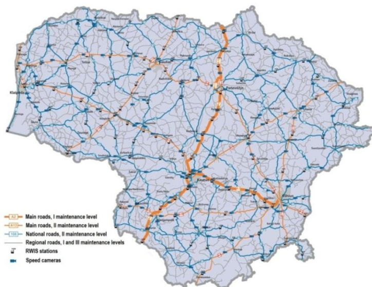
Fig. 3. Map of winter road maintenance according to maintenance levels
