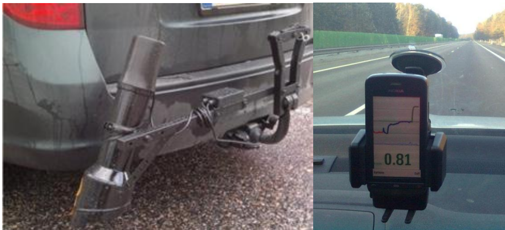
Fig. 4. Mobil optical friction measurement device RCM 411 (on the left) and user's interface (on the right)
