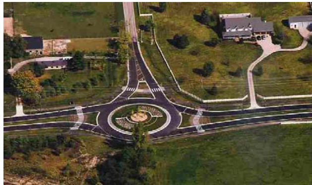
Photo 1 - A small-scale single-lane roundabout in a suburban area of the United States
