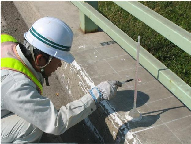
Photo 6 - Measurement of the water permeation ratio
