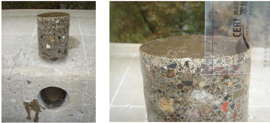
Photo 13 – The wetted core (The layer near the upper surface that is not wet is the water-repellent layer.)
