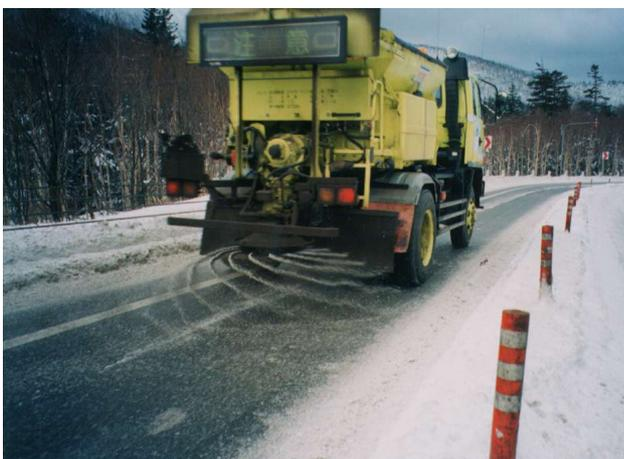
Photo 1 - Deicing salt spraying
