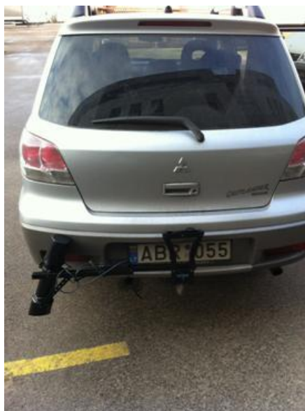
Figure 6 – A sensor for measurement of friction (RCM 411) installed on a tow-ball of the vehicle
