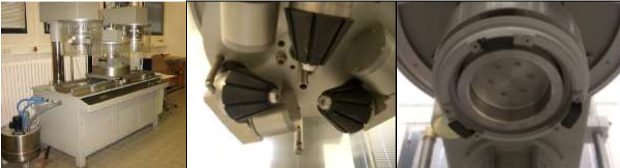
Figure 4 – Wehner/Schulze machine (left), the polishing unit (middle) and the skid resistance measuring unit (right)
