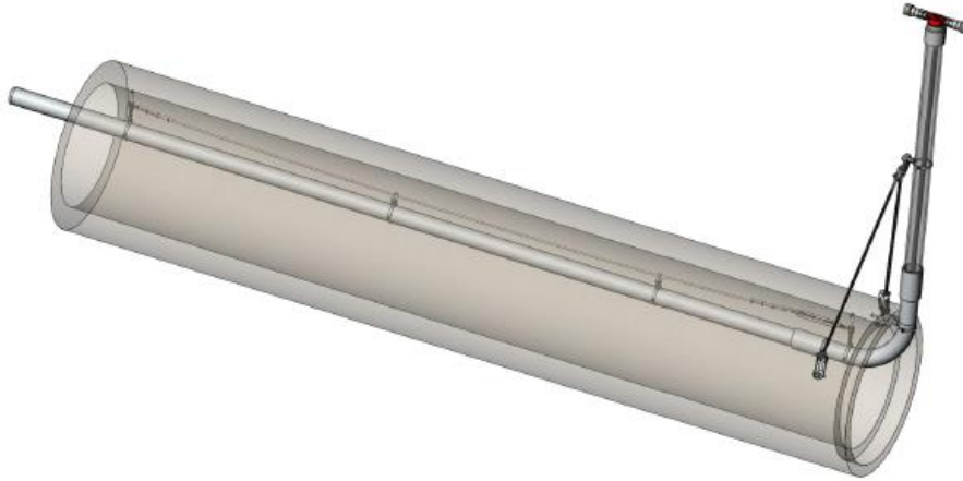
Illustration 3 – IGS mounted in culvert Source: Heatwork
