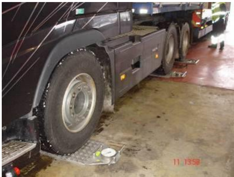
Figure 9 - Set-up for weighing with mobile scales
