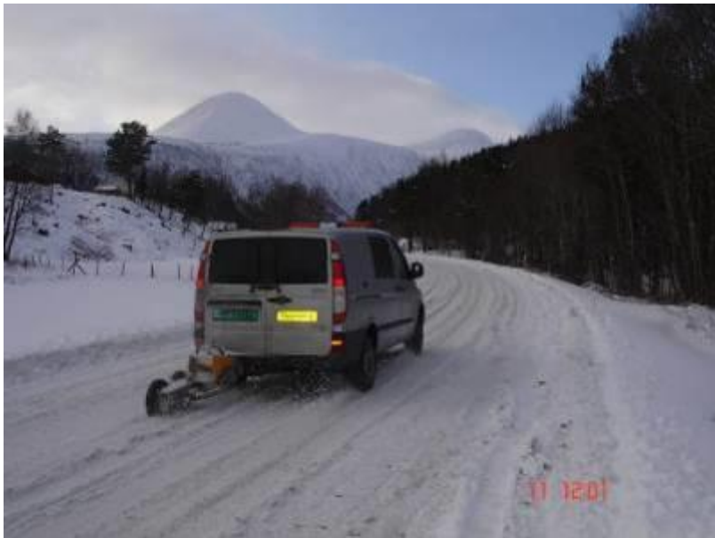
Figure 10 - Friction measurement with the type TWO friction trailer
