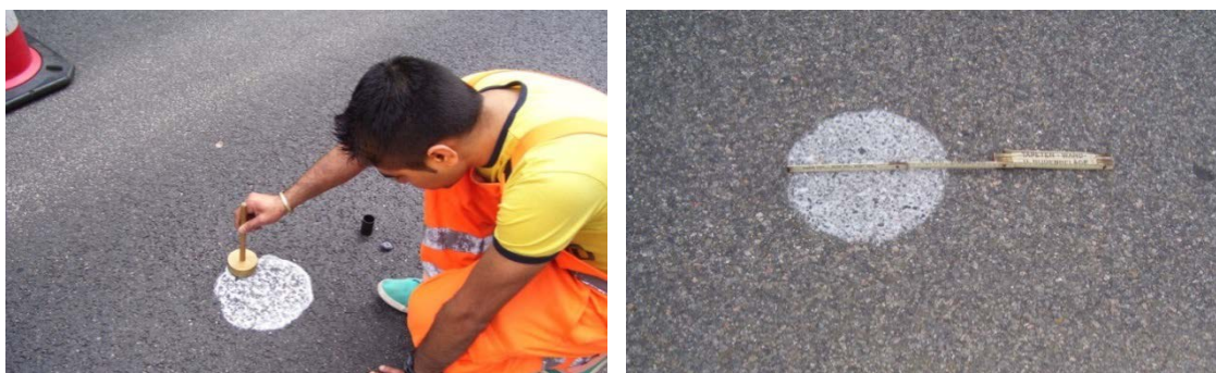
Figure 3 – Determination of mean texture depth with the sand patch method
