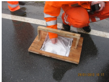
Figure 2 – Towel test on wet road surface
