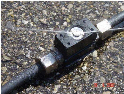
Figure 8 - Spay head of FAST-System (left) and situation after spraying at Bern-Wankdorf in Dec. 2012 (right)
