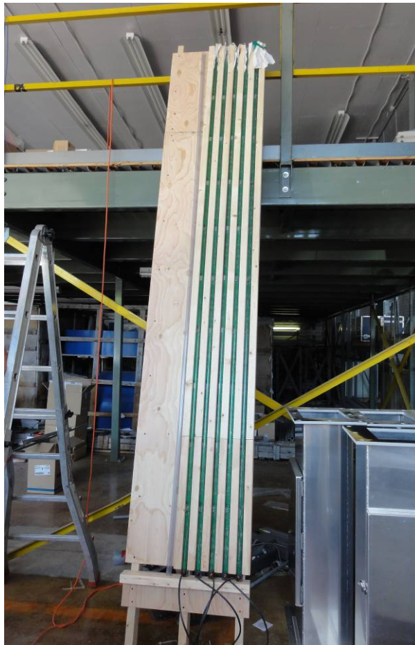
Figure 9 - Support de fabrication des tubes de gel
