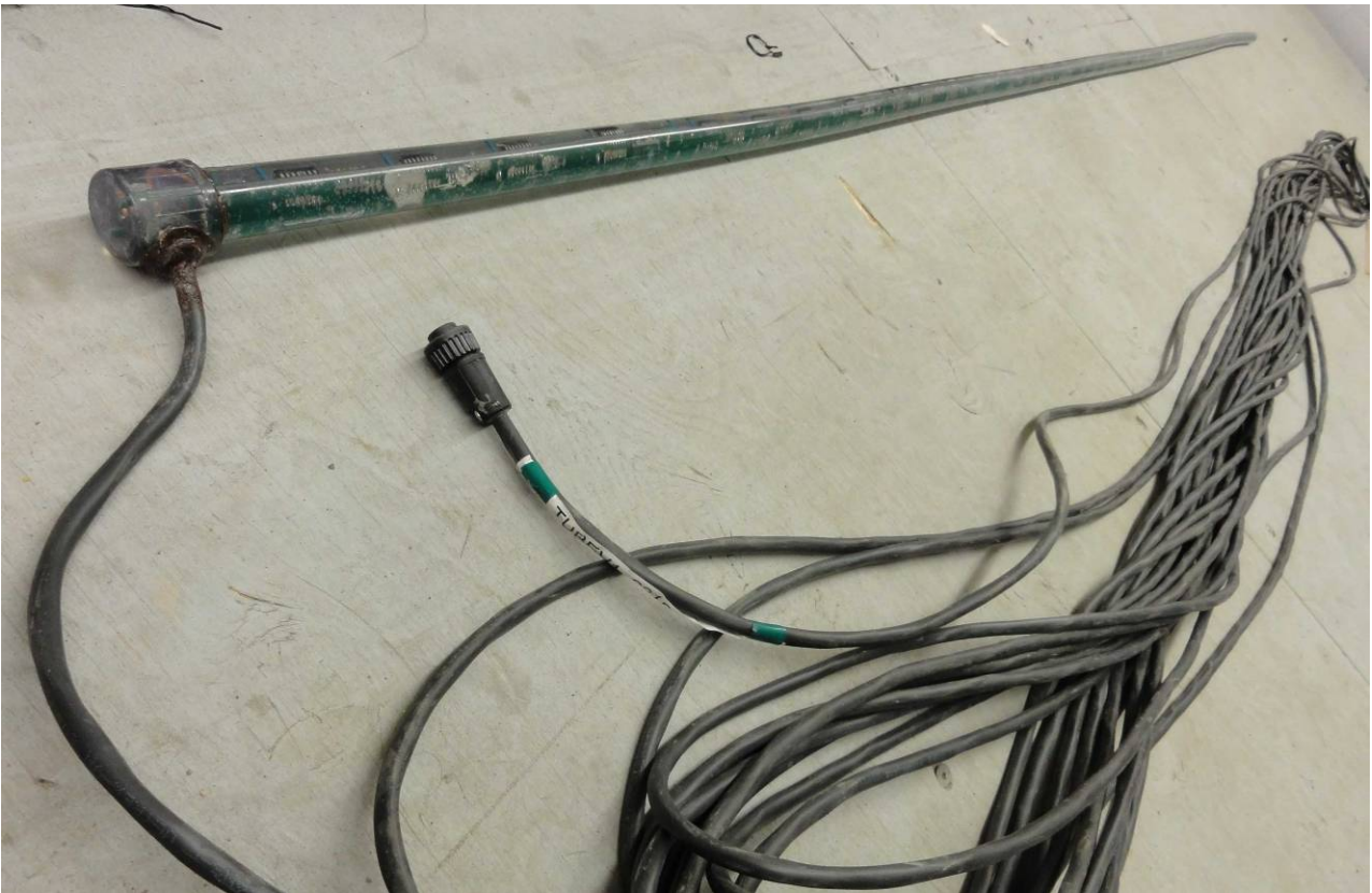
Figure 3 – Frost probe with automated reading
