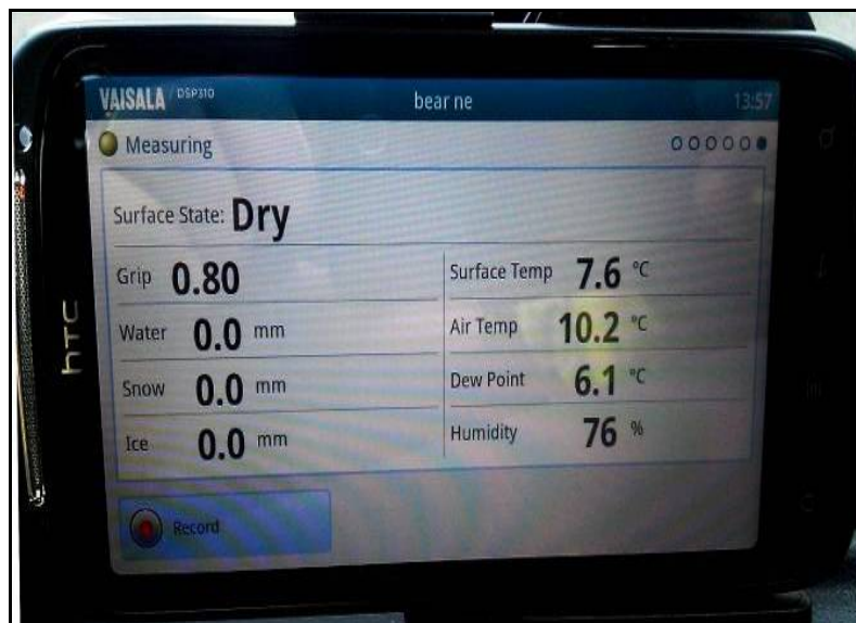
[Figure 7 – Mobile Sensor Output as seen by the Winter Service Patrol Driver]
