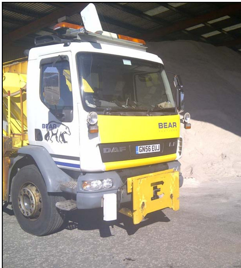
[Figure 6 - Vaisala DSP310 Condition Patrol Installed on Winter Patrol Spreader]
