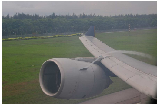
Figure 21 - Condensation vortices from a nacelle strake at takeoff.
