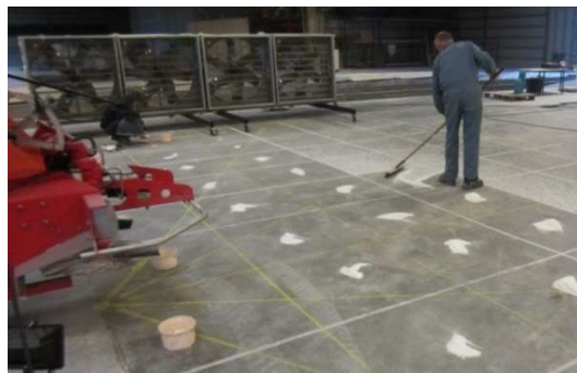
Figure 1 - Manual collection of salt deposited on each test square.
