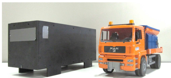
Figure 13 - The scale model of a salt spraying truck and the simplified box model with the same outer dimensions.
