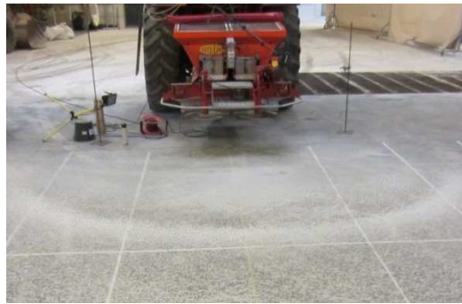
Figure 3 - Salt distribution from the stationary spreader at no crosswind.
