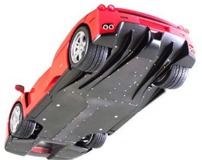
Figure 24 - Example of a paneled underbody and rear diffuser on a car.
