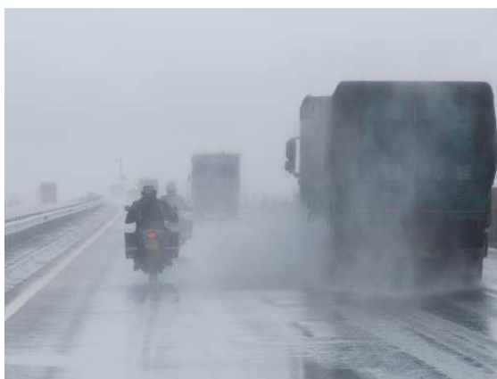
Figure 12 - A truck creating turbulence and discharging water droplets and mist to the sides and backwards.
