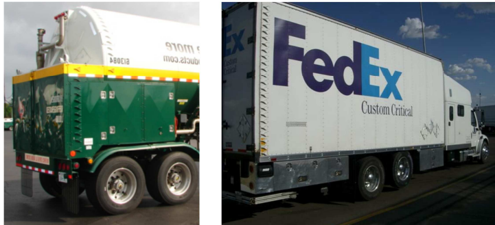
Figure 25 - Vortex generators installed on the rear facing surface of a tanker and a trailer.
