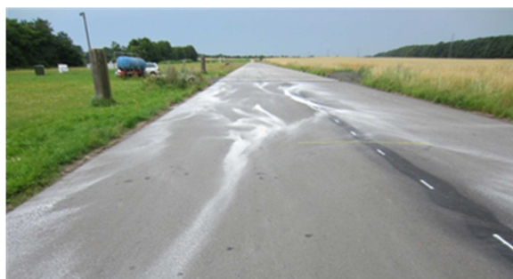
Figure 9 - Salt distribution patterns after passage of salt spreader truck.
