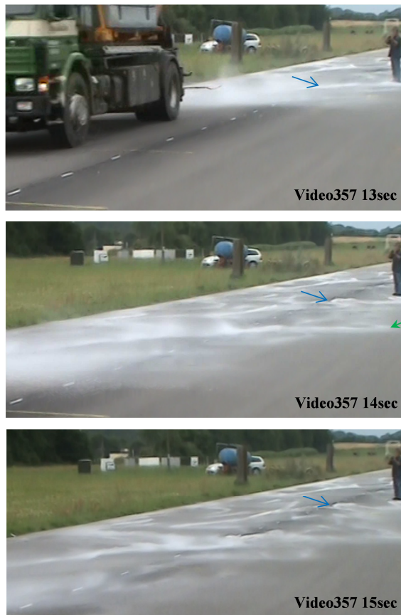
Figure 11 - Development of salt spreading during passage of the truck.
