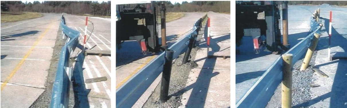
Figure 2: quasi-static loading test (from left to right: steel post, plastic post and wooden post)
