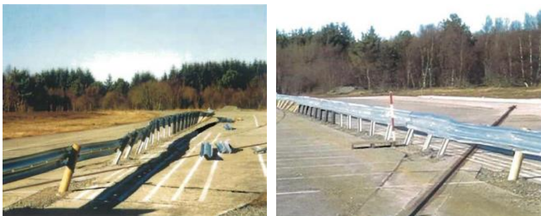
Figure 3: result of snow clearing simulation test
