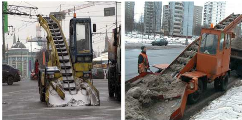
Figure 2 - Snow removal equipments for collecting snow along the road
