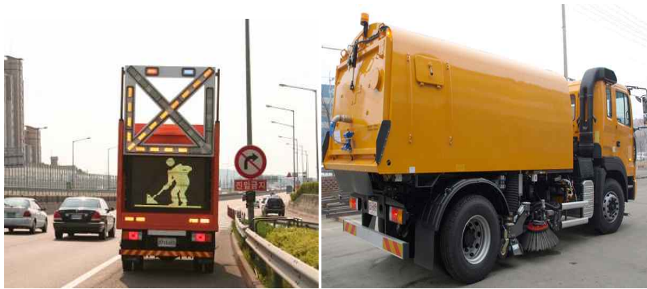
Figure 5 - Type of equipments used for road maintenance work in off-winter seasons
