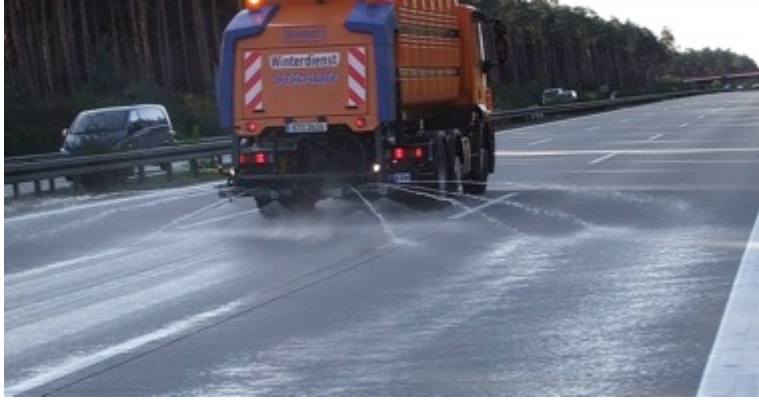
Figure 6: Schmidt liquid spreading machine with a set spray density of 40 g/m 2 and spray width of 11.25 m
