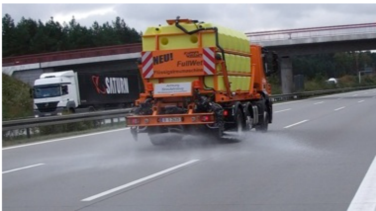
Figure 5: Küpper-Weisser liquid spraying machine with a set spray density of 20 g/m 2 and spray width of 7.50 m
