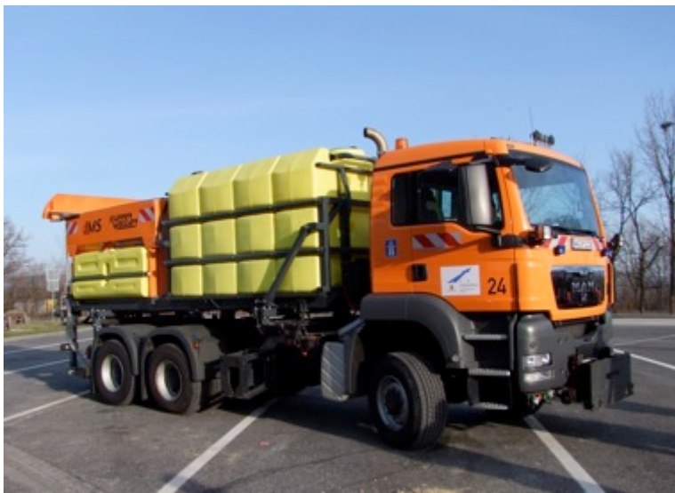
Figure 7: Combination spreading machine from Küpper-Weisser for 10000 l brine and 5 cbm dry salt
