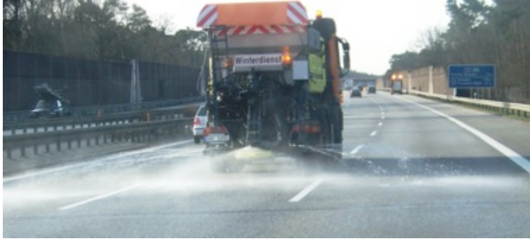
Figure 3: Küpper-Weisser combination spreading machine with a set spray density of 20 g/m 2 and spray width of 11.25 m
