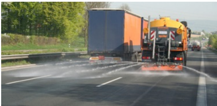
Figure 4: Epoke liquid spreader with a set spray density of 20 ml/m 2 and spray width of 11.00 m
