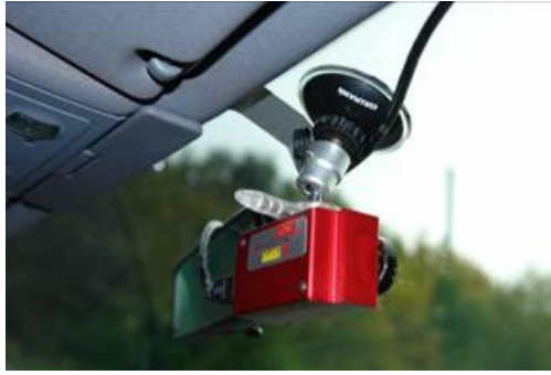
Figure 6 Road surface monitoring system with a stereo camera (by Finland)
