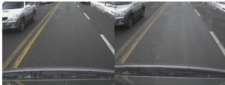
Figure 11 Brightness difference for wet road surface condition with stereo camera:
