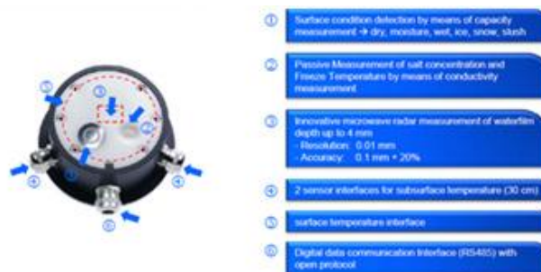
Figure 1 Ground embedded road surface state sensor (by Lufft, Germany)
