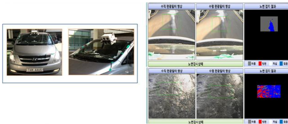
Figure 13 Probe-car based mobile road surface monitoring system concept
