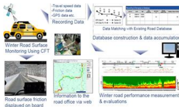
Figure 3 Winter road maintenance system with CFT (by CERI, Japan)
