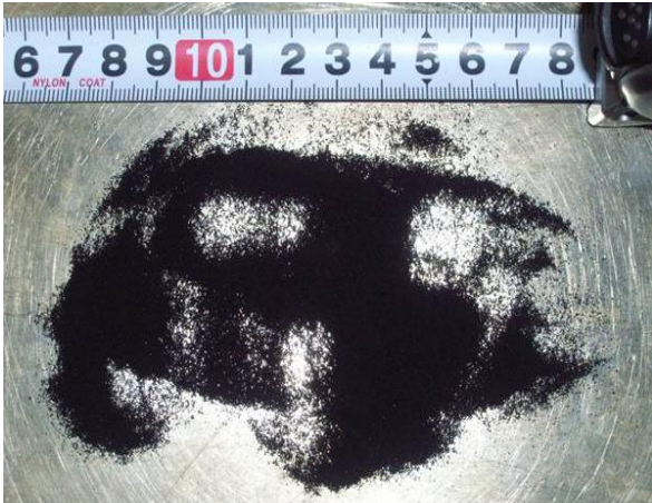
Photo 1 Rubber powder (Particle diameter: 0.3 mm or less)
