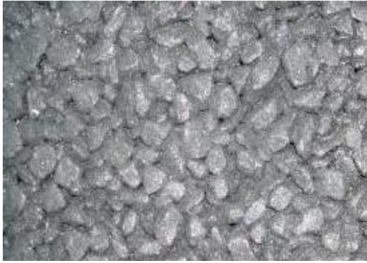
Photo 7 Surface of drainage pavement after application of rubber powder
