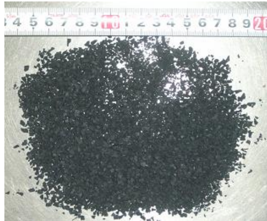
Photo 2 Rubber chips (Particle diameter: 1 to 5 mm)
