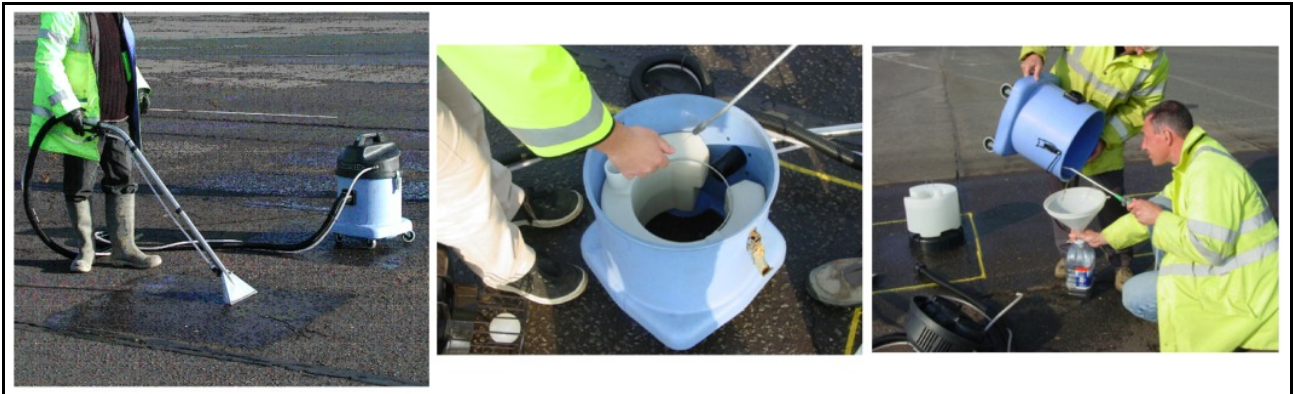
Photograph 1 - Salt recovery using wet-wash method
