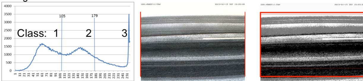
Figure 1 - Histogram and classes. The left figure is the pixel intensity histogram and the threshold value solved from the discriminant analysis for three class. The histogram was made from the center image. The third image from the left is a post-processed, three intensity value (black, gray, white) image using the threshold values.
