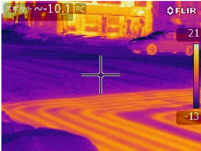
Figure 2 - Road intersection with installed heater
