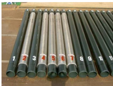
Well screen pipes
