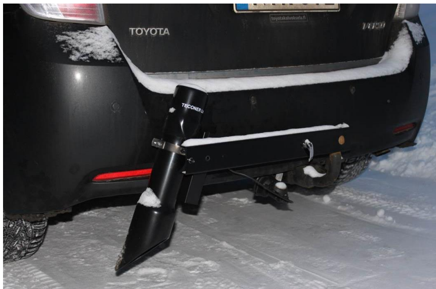
Figure 1. RCM411 installed by a trailer ball joint adapter.
