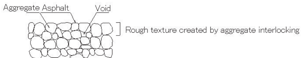
Figure 2 - Cross-section of drainage pavement [5]
