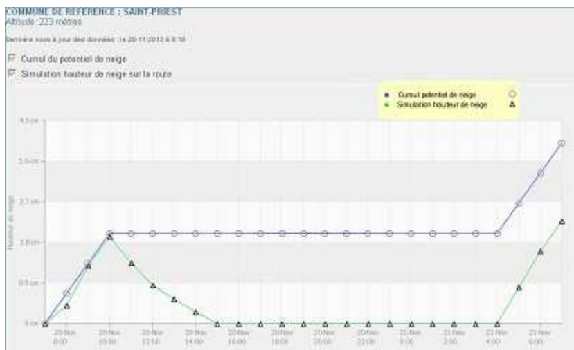
Graph 1 – Snow depth on the road (green) and cumulative snow potential (blue) in Saint-Priest
