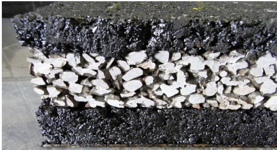
Figure 5 – test specimen with PUR-interlayer (detail)
