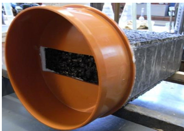
Figure 9 – Water supply sleeve at the front side of the prototype
