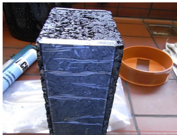
Figure 8 – test specimen sealed at the side
