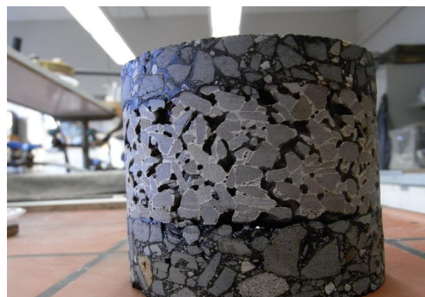
Figure 19 – Visual appearance of the PUR interlayer test specimen after the test
