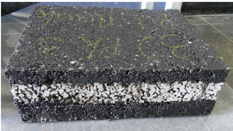
Figure 4 – test specimen with PUR-interlayer
