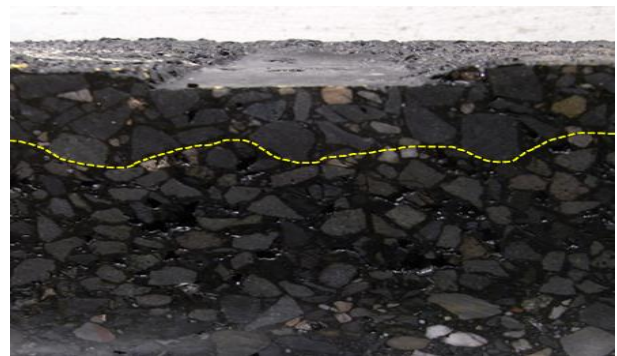
Figure 15 – displacement between surface layer and PA interlayer
