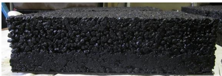
Figure 6 - test specimen with bituminous interlayer PA 8
