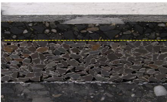
Figure 14 – no material displacement between surface layer and PUR interlayer
