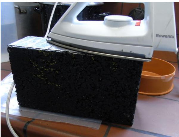
Figure 7 – sealing the sides of the test specimen with bitumen tape and iron
