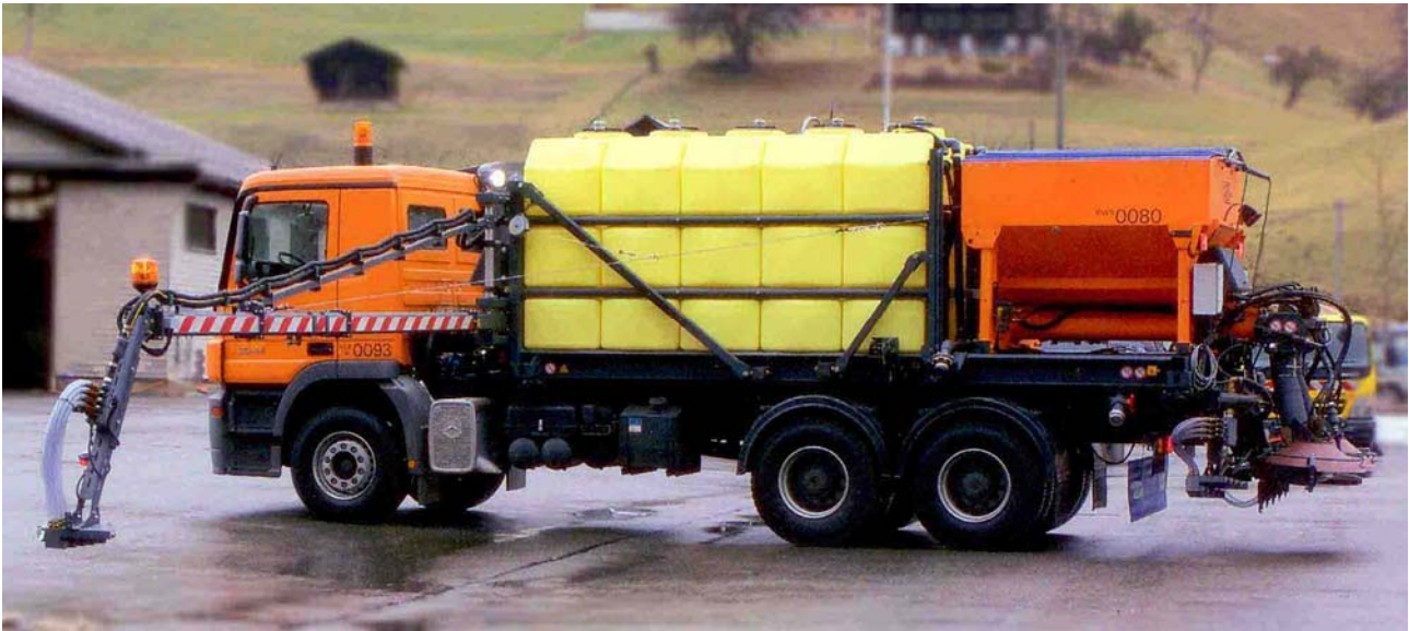
Photo 4 – Image of the “COMBI”-type melter spreading equipment
