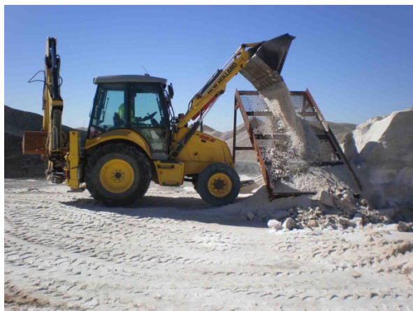
Photo 6 – Sifting the NaCl remaining from one winter road management campaign.
