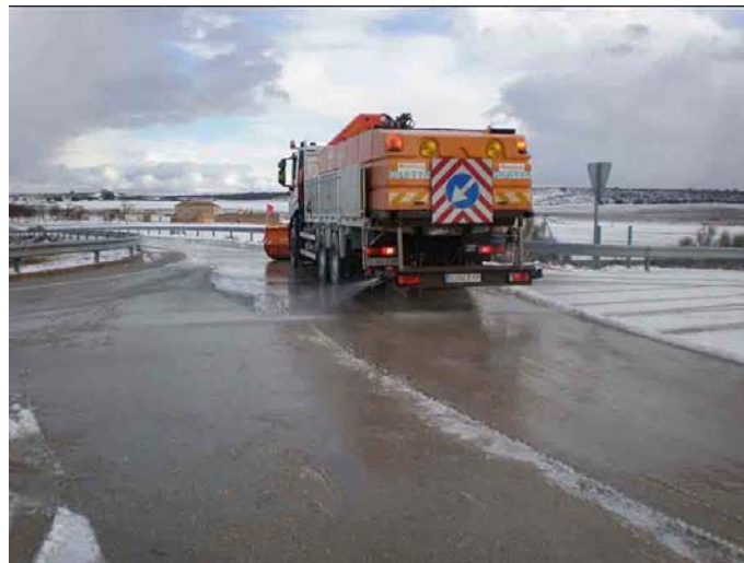
Photo 3 – Spreader of liquid state melters
