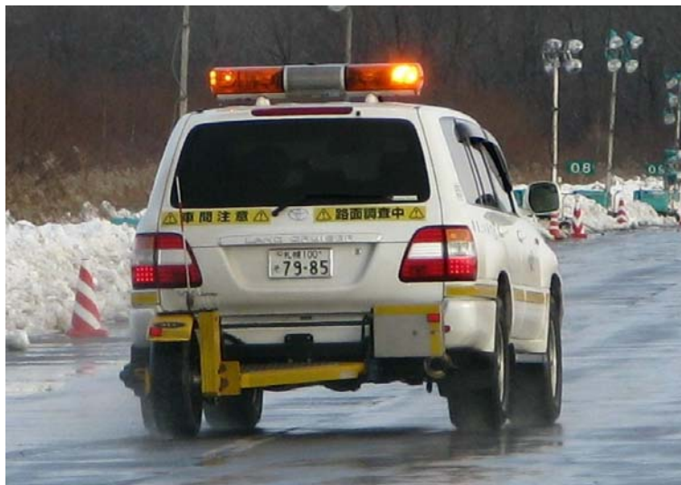
Figure 2 - Continuous friction tester (CFT)
