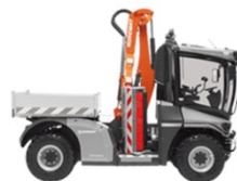
Fig. 12.3.a - Dedicated equipment-carrier with integrated grass/brush-cutting arm able to be fitted simultaneously with three different equipment
