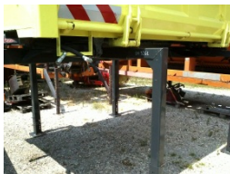
Fig. 7.2 - Spreader on supporting legs after removal
