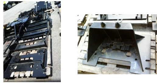
Fig. 9.2 - European plate integrated to several different coupling systems
