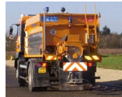
Fig. 4 - Spreading up to 2 lanes with a disc
