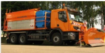
Fig. 1 - Front brine tank of a mixed machine
