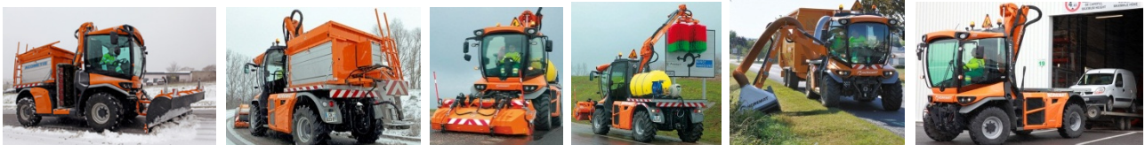
Fig. 12.3.b - Dedicated equipment-carrier for road operation
