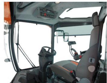
Fig. 11.2 - Cab redesigned to improve visibility and ergonomic of the control station
