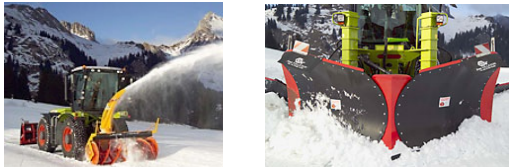
Fig. 12.1 - Dedicated equipment-carrier for snow blower, wedge-shaped snow plough, side plough or huge grass-cutter
