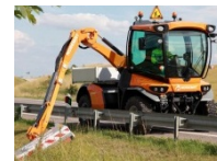
Fig. 12.3.a - Dedicated equipment-carrier with integrated grass/brush-cutting arm able to be fitted simultaneously with three different equipment
