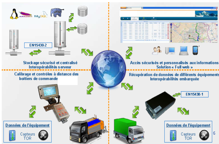
Fig. 15 - An open and adaptable architecture fulfilling European standards
