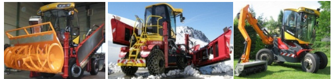
Fig. 12.2 - Dedicated equipment-carrier for snow blower, wedge-shaped snow plough, spreader, branch pruning of grass-cuter
