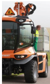
Fig. 11.1 - Safe access from the rear of the cab via a standing platform in the size of the carrier
