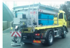
Fig. 2 - Lateral brine tank of a mixed machine
