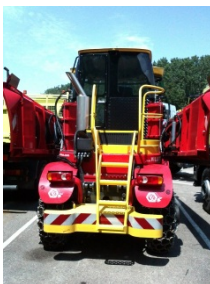
Fig. 11.1 - Safe access from the rear of the cab via a standing platform in the size of the carrier
