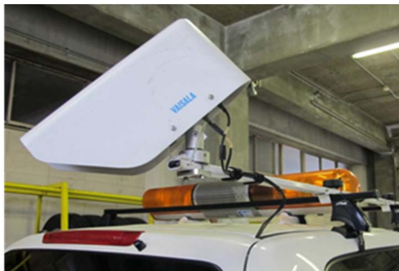
Photo 4 - Non-contact sensor utilizing infrared rays
