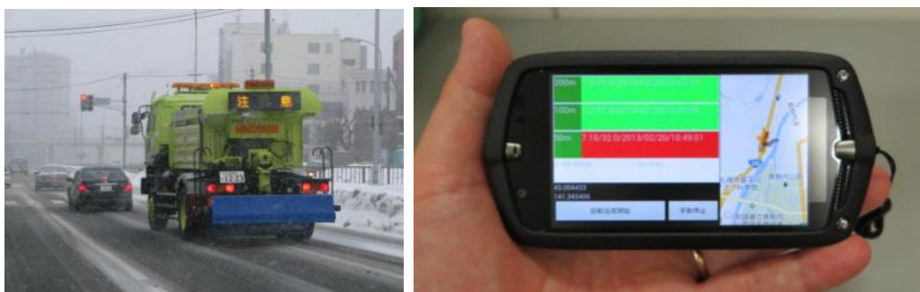
Photo 6 - Friction monitoring data provided to operators on the spreader trucks
