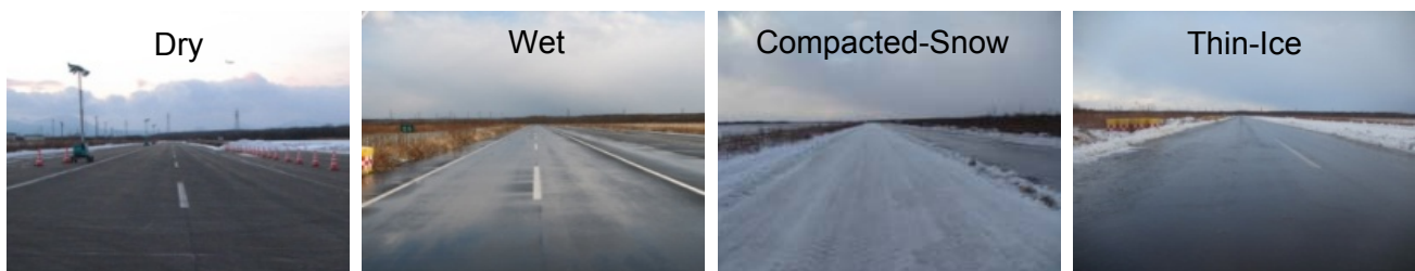
Photo 5 - Surface conditions prepared in the test track
