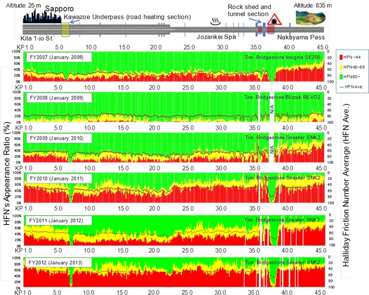
Figure 6 - Appearance ratio of different road surface conditions and HFN values on NH230 (January, 2008~2013)
